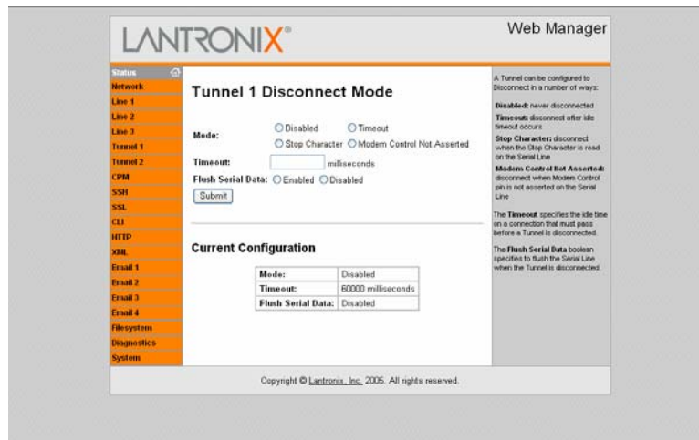
Figure 4-17. Tunnel 1 Disconnect Mode
